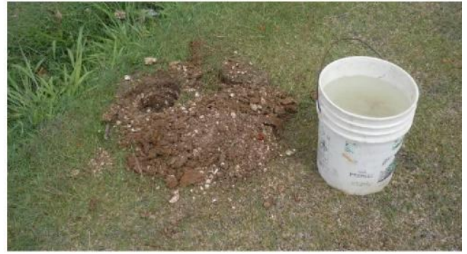
Dig a hole and test the soil infiltration rate.
