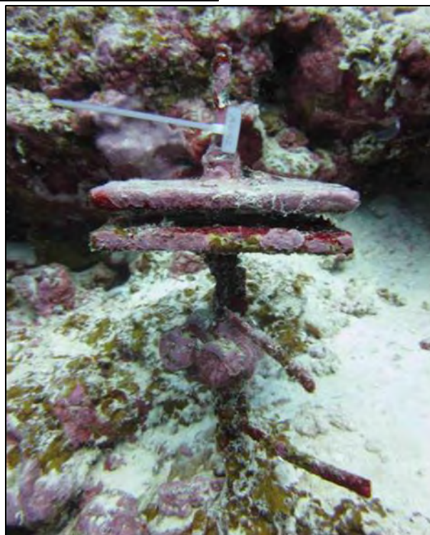
Figure A-18 Calcium acidification unit pre-deployment and two years after deployment
