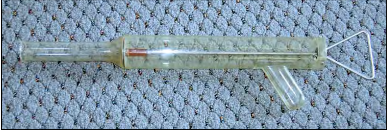
Figure A-13 Slurp gun
