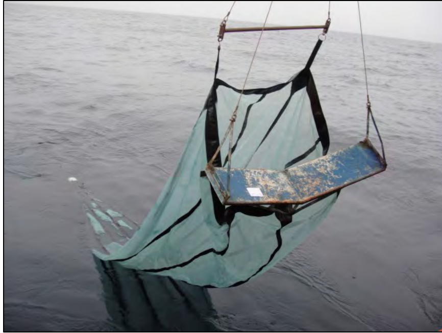
Figure A-3 Isaacs-Kidd 6-ft trawl
