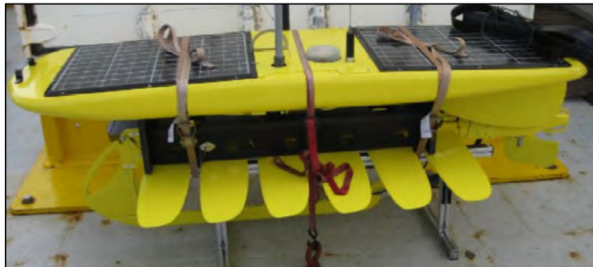
Figure A-24 Oceanographic glider
