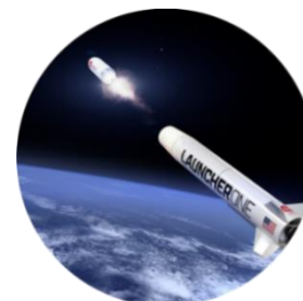
First and Second Stage Separation
