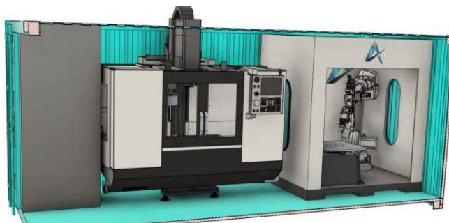
Figure 15: Highlights single 40-foot Connex equipped with portable robotic AM cell, CNC mill, and heat treatment furnace. (Source: ADDITEC, Fabricating & Metalworking)
