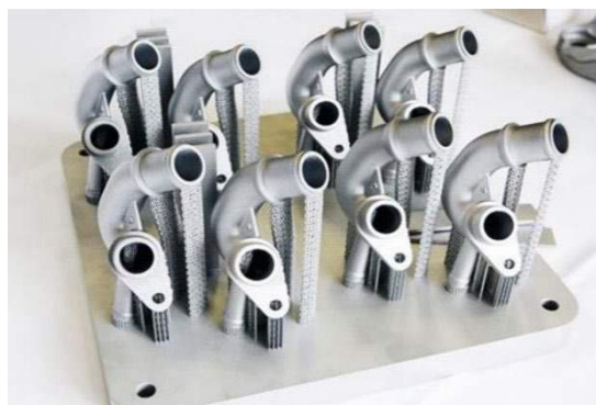
Figure A15. The metal water connectors for AUDI W12 engine were 3D printed on demand. Credit: AUDI
