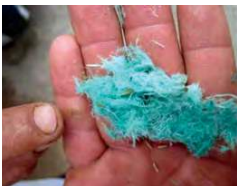
The hydroseed mix is a combination of seed, paper or wood fiber mulch, binder (tackifier) product, and sometimes fertilizer.
