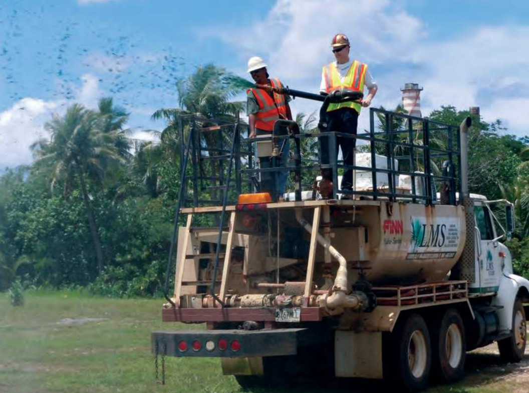
Hydroseeding truck includes a mixing tank and dispersal cannon and hose.
