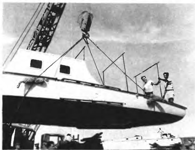
FIGURE 16.—SES 800. Note glass ports near stern. Propulsion is by an outboard motor.
