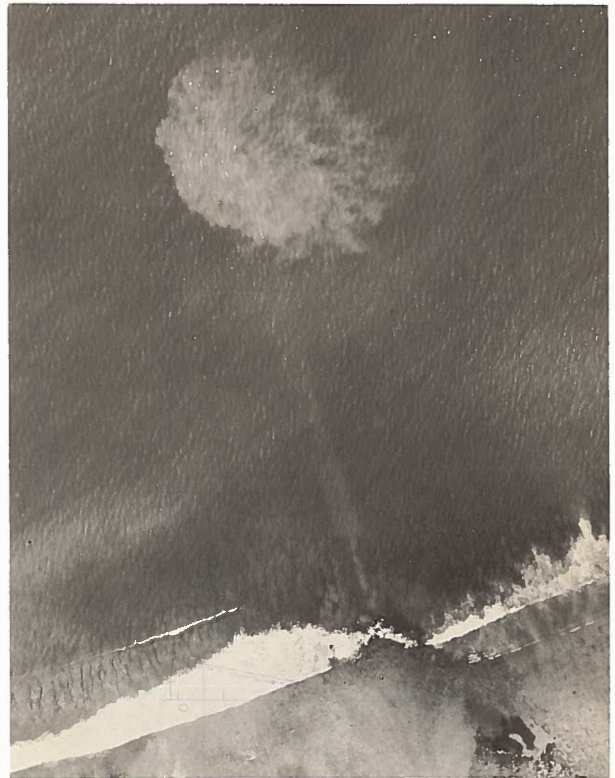
Figure 22. AERIAL PHOTOGRAPH OF SEWAGE "BOIL". A pumping cycle has just started. Note the track of the outfall main through the reef margin and across the submarine terrace, (Photograph through the courtesy of Navy Heavy Recon. Squadron VAP-61, now VQ-1).
