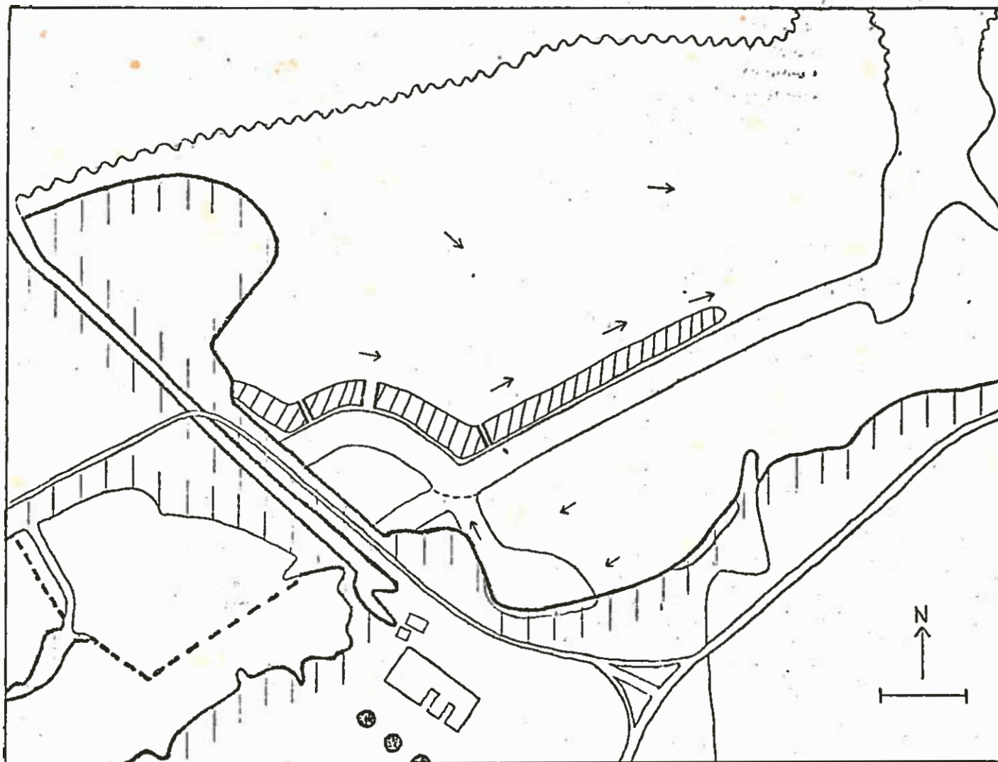
Figure 5. General current patterns in West Piti Bay with the construction dike extending approximately halfway along Tepungan Channel. The length of the arrows is roughly proportional to the flow velocity. Note the placement of culverts and passes in the dike.
