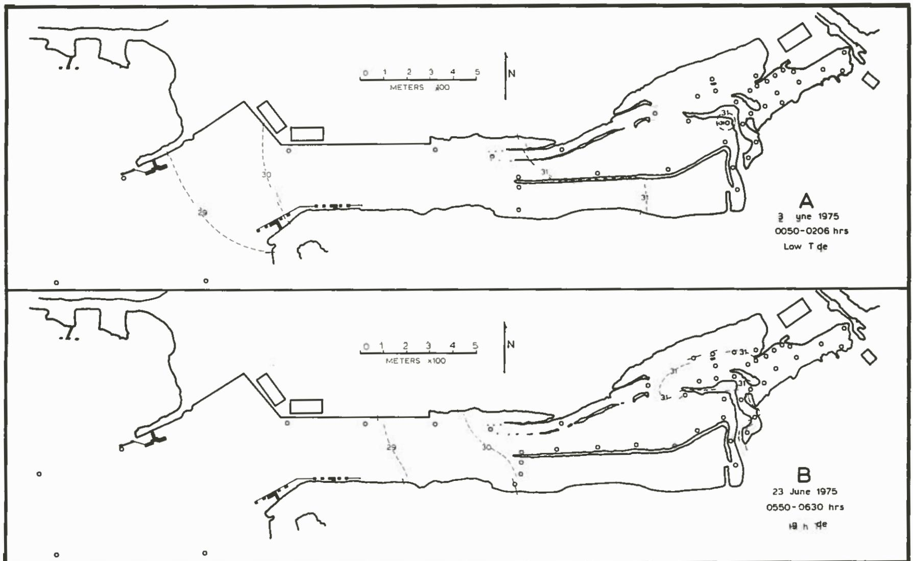
Figure 9. Surface temperatures in the Piti Channel area during low and high tides on 23 June 1976. A. During a low tide predicted to be +1.6 ft. at 0106. B. During the following high tide predicted to be +2.4 ft. at 0651.
