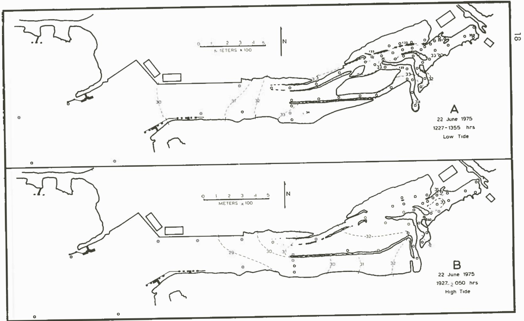
Figure 8. Surface temperatures in the Piti Channel area during low and high tides on 22 June 1975. A. During a low tide predicted to be -0.4 ft. at 1251. B. During the following high tide predicted to be +2.4 ft. at 2015.
