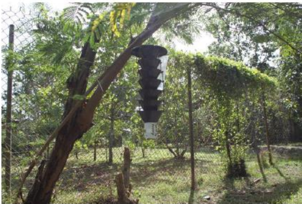
Funnel trap installed to monitor for insects and test early detection tools.
