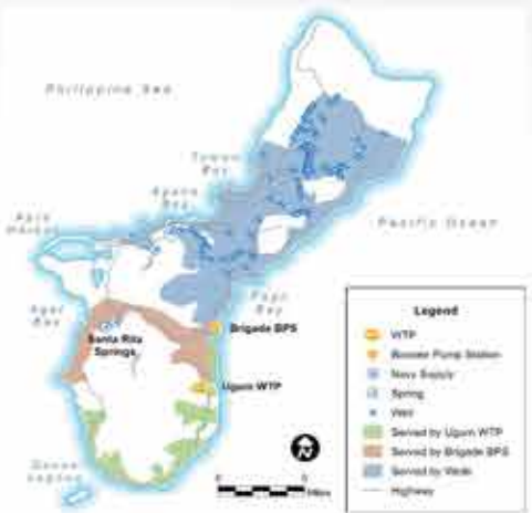
Hydraulic Model – Island-wide water distribution system
