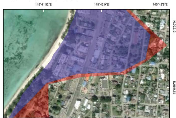
This map shows the simulated flooding for 100-year storm events with (blue) and without (red) coral reefs in Saipan, CNMI.
