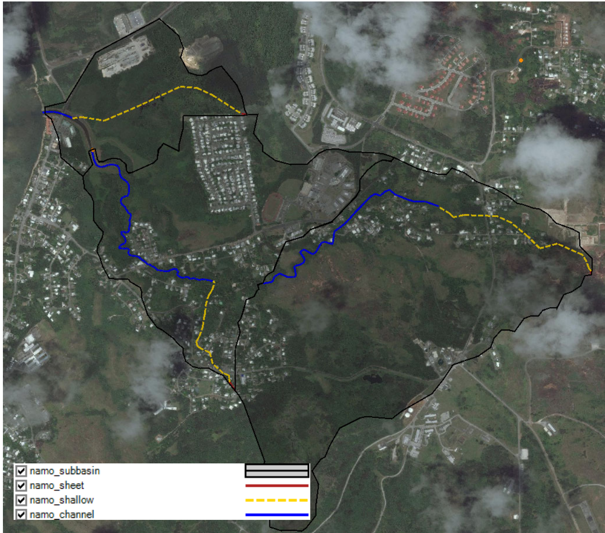
Figure 4-2: Sheet Flow, Shallow Concentrated Flow, and Channel Flow Delineated, Namo River, Agat Watershed
