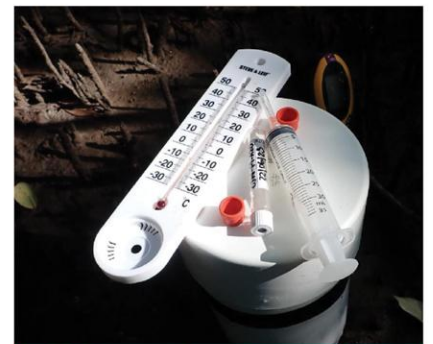
Equipment used to collect greenhouse gases emitted from mangrove sediments. Research like this enables scientists to better understand how efficiently carbon is stored and informs climate change policies.
