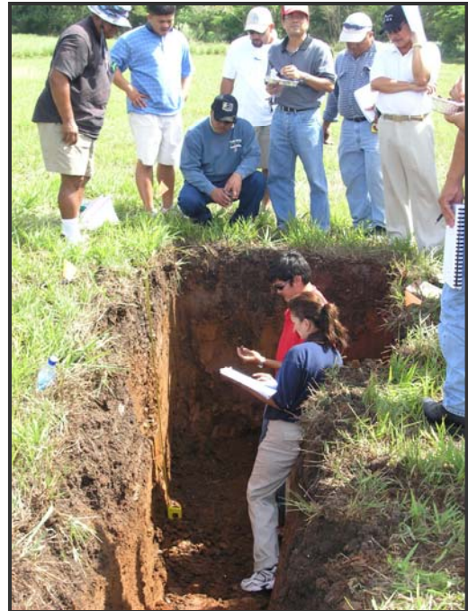
Figure 8.3 Participants of the May 2006 Stormwater Training Workshop in Saipan learn how to evaluate a test pit.
